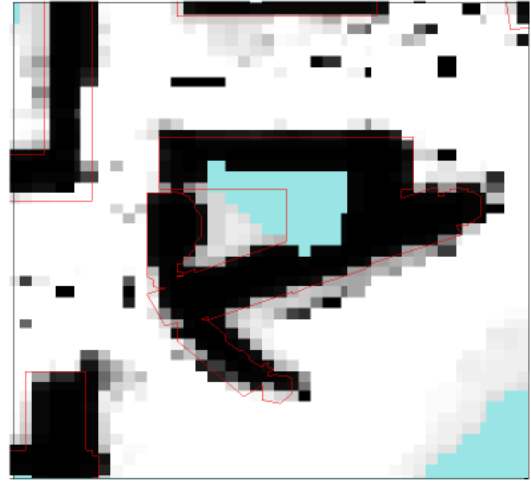
Fig. 6. The horizontal slice (3-6 meter height) of the relevant portion of the prior map of UCSB campus used in experiments. Cells with high/low probability of occupancy are colored with black/white. The red lines indicate building boundaries according to Open Street Maps.
