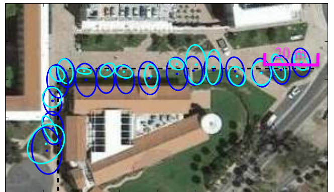
Fig. 7. The resulting geo-location improvement from Algorithm 1. The blue ellipses represent geo-location reported by the GNSS receiver. The cyan ellipses represent the geo-location estimates resulting from the Algorithm 1. The black dashed line represents ground truth of the GNSS receiver trajectory.
