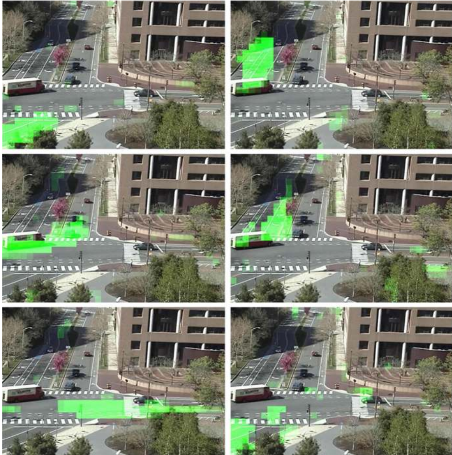
Fig. 6 Illustration of our learned factors overlaid with data the from MIT dataset. The left column presents three common patterns. Three rare factors are displayed in the right column
