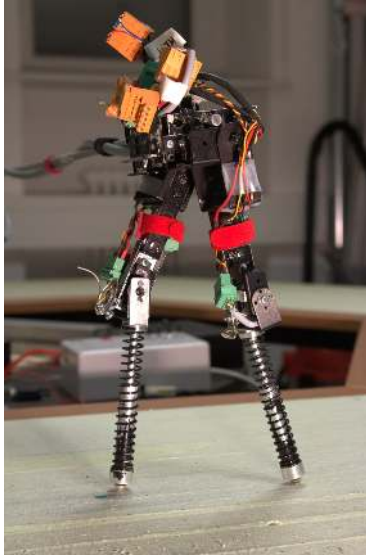
Fig. 1: The bio-inspired dynamical bipedal walker Fox . Using Bayesian optimization, we found reliable and fast walking gaits with a velocity of up to 0.45 m/s.
