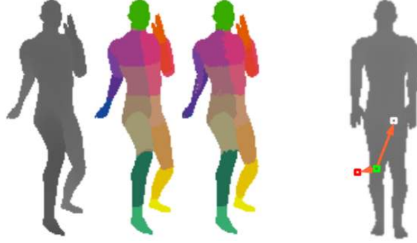
Figure 5. Left: ground truth depth, ground truth body parts and predicted body parts; Right: features specified by offsets u and v .
