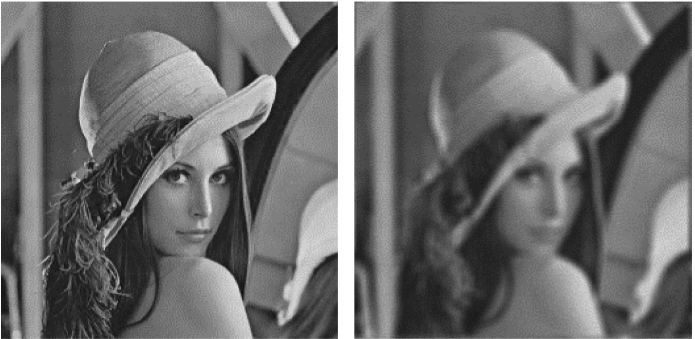
Fig. 1. (a) Original “Lena” image. (b) Degraded “Lena” image with 7 \times 7 uniform blur and additive noise SNR = 25.36 dB.
