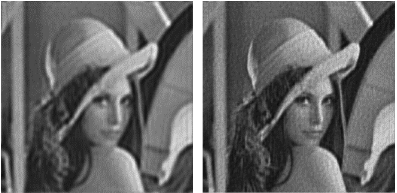
Fig. 1. (Continued.) (c) Wiener filter restoration, ISNR = 3.2 dB. (d) “Optimal” Wiener filter restoration, ISNR = 4.40 dB.
