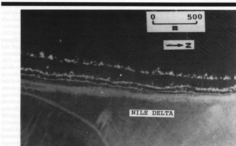
Figure 3. Vertical aerial photograph at the eastern side of Abu Quir Bay showing the three shore parallel bars as indicated by wave breaking. Note the three lines of wave breaking alignment to the shoreline.
