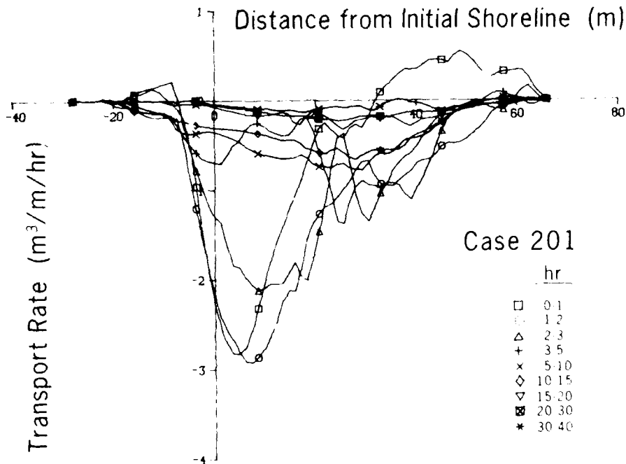
Figure 17. Time evolution of net cross-shore sand transport rate distribution for Case 201, accretionary case
