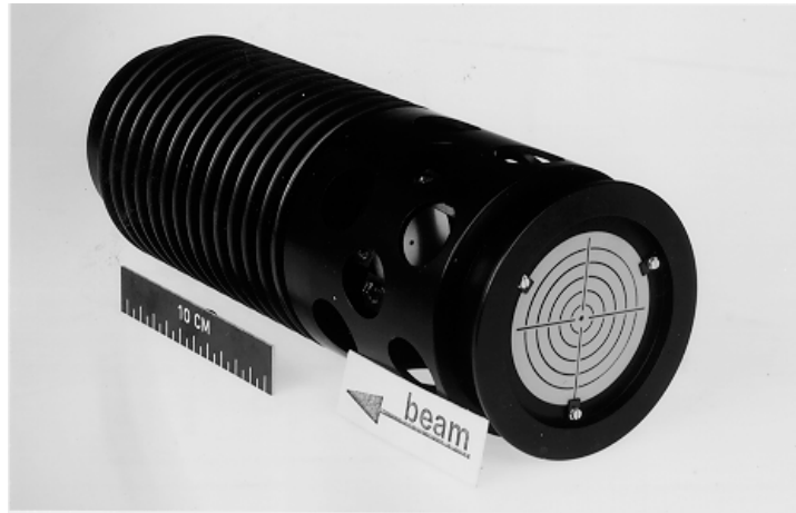
Fig. 25 Scintillator plate mounted on the antiproton production target of the CERN Antiproton Accumulator.
