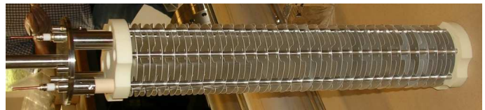
Fig. 2. Photograph of the inside of an ionization chamber. The stack of aluminum electrodes with the insulator ceramics at both ends can be seen.
