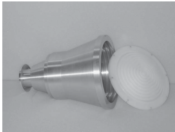
Figure 10. Photograph of the 7.25 GHz corrugated conical horn and the hyperbolic-planar lens.
