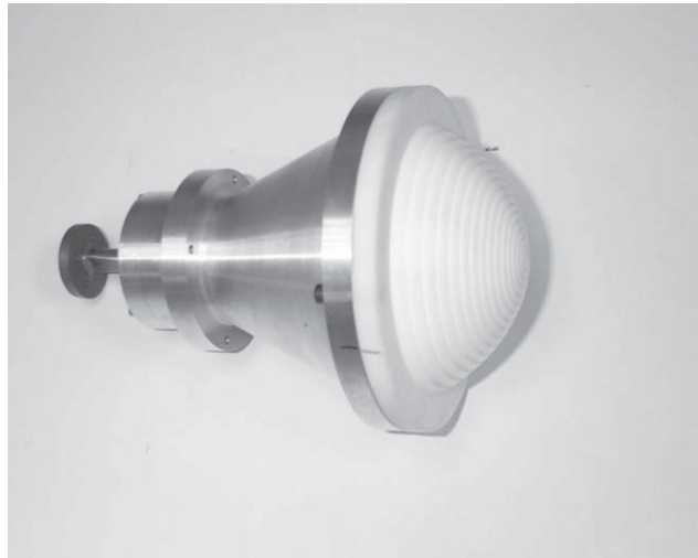
Figure 16. Photograph of the 30 GHz corrugated conical horn and the spherical-elliptical lens.
