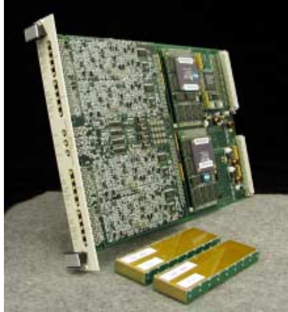
Figure 2. Four-Channel AFE Module With Two of the Four Battery Units Shown
