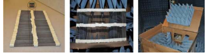
Fig. 3. Measurement setup for acquiring the S-parameters of the unit-cell array.
