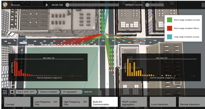
Figure A.4: Visualisation example of communication between cars.
