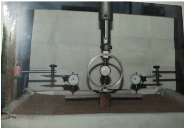
Fig. 2 Loading arrangements for load tests in a square test tank
