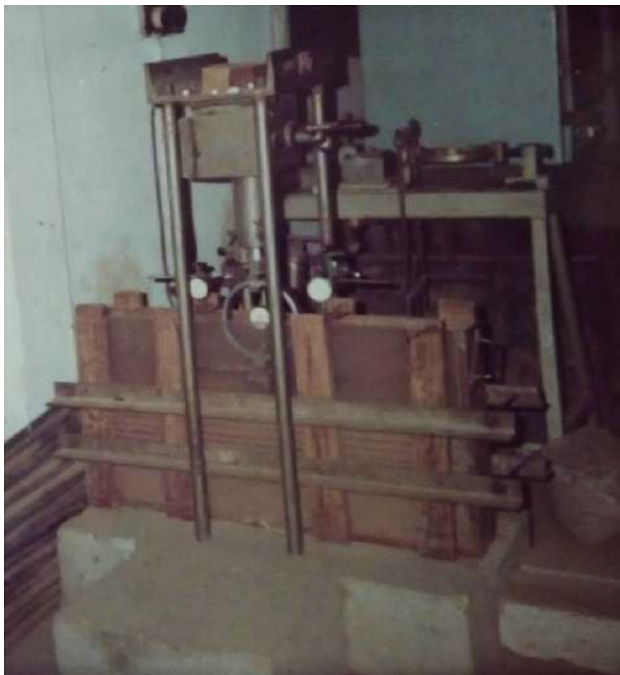
Fig. 12 Loading arrangements for load tests in a rectangular test tank
