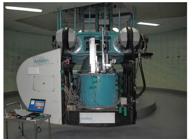
Fig. 1. Centrifuge equipped with a test-ready model of this study
