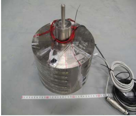
Fig. 4. Model bucket foundation
