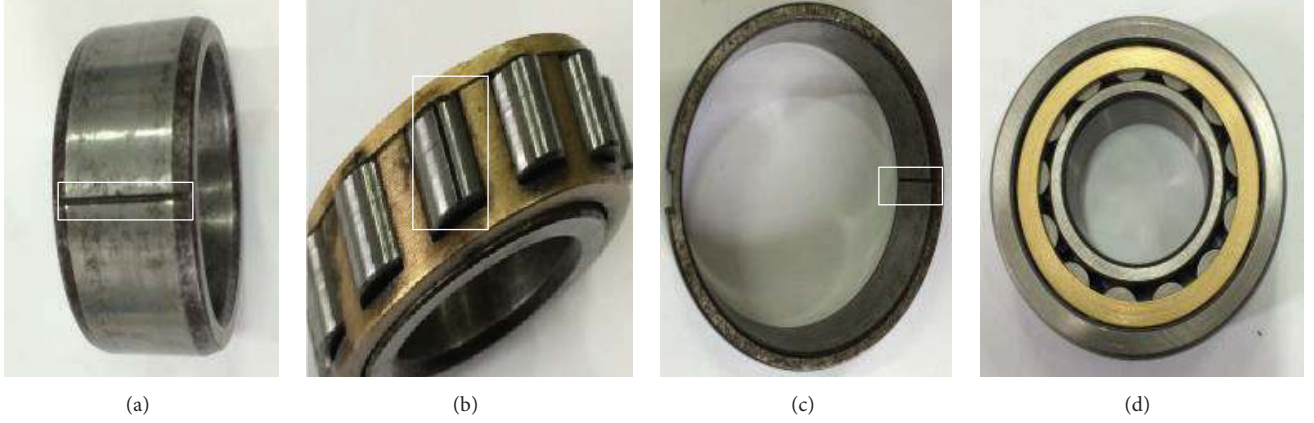
FIGURE 5: Pictures of the testing bearings: (a) inner race fault; (b) ball fault; (c) outer race fault; (d) normal.
