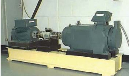
FIGURE 3: Bearing test rig of Case Western Reserve University Data Center.
