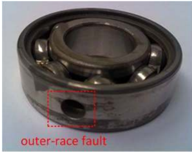
Fig. 12. Test bearing with an outer-race fault.
