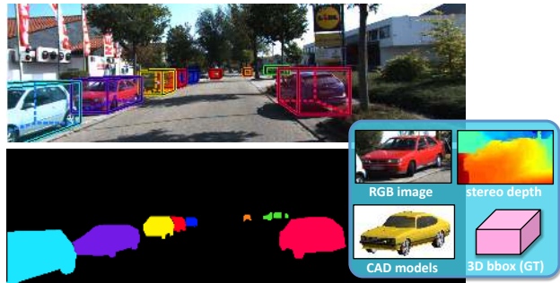
Figure 1: Our goal is to automatically generate segmentation ground-truth (bottom) using weak labels (top image).
