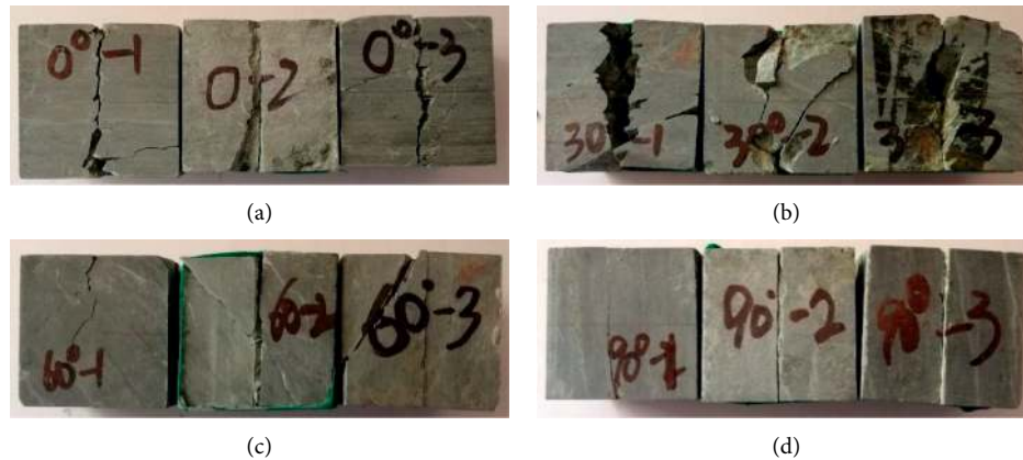
FIGURE 11: Variable angle shear failure diagram with different bedding orientations: (a) \beta = 0^\circ ; (b) \beta = 30^\circ ; (c) \beta = 60^\circ ; (d) \beta = 90^\circ .
