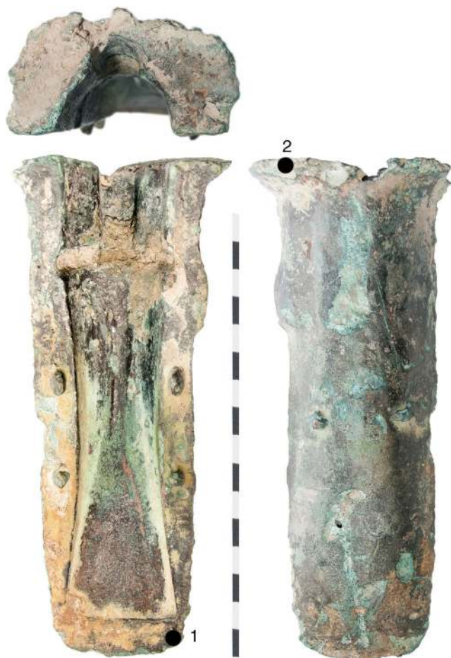
Fig. 2 Metal casting mould from Gaj Oławski in southwestern Poland. The numbers refer to sampling locations. On the right side, heavy corrosion marks and two small knobs are visible. Photo by Ł. Kapa
