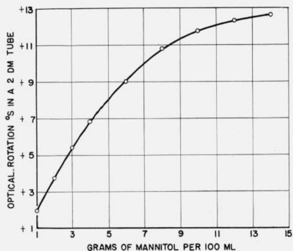
FIGURE 12. Optical rotation of mannitol in the presence of 10 g of Na_2B_4O_7 \cdot 10H_2O per 100 ml of solution.
