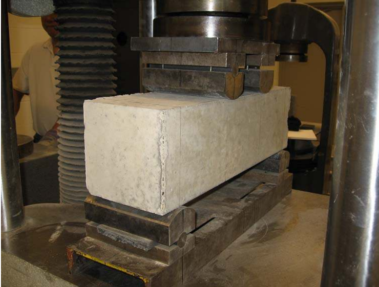
Figure 3-15 Flexural test to obtain the modulus of rupture
