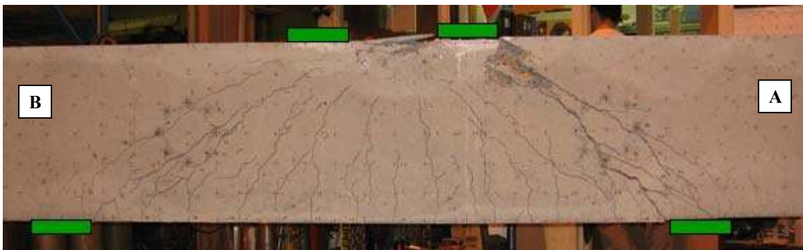
Figure 4-26 Specimen MS2-3 after failure
