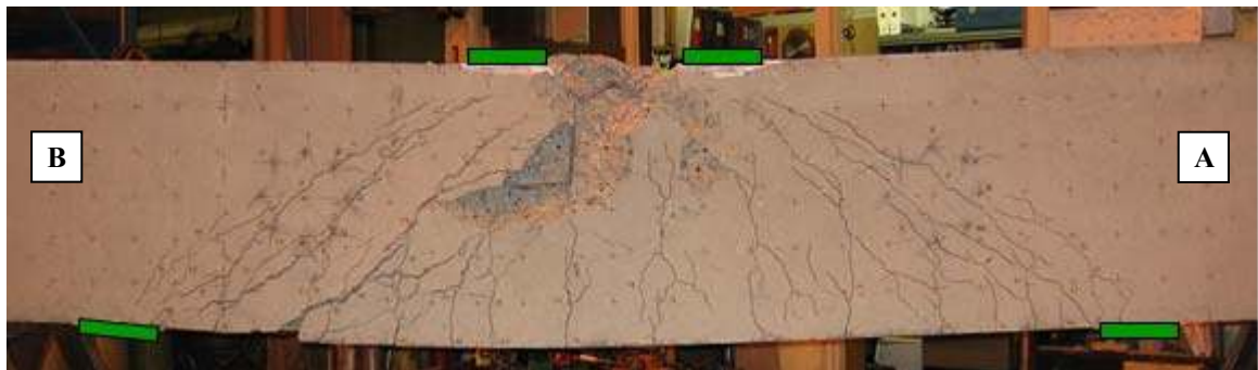
Figure 4-20 Specimen MS2-2 after failure
