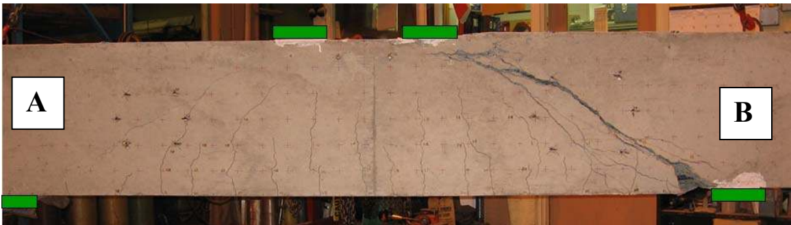
Figure 4-44 Specimen MW3-2 after failure
