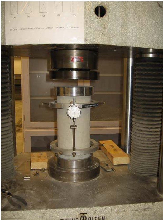
Figure 3-14 Compression test of concrete cylinder
