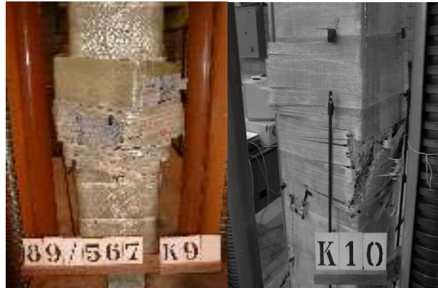
Fig. 2 Confined concrete columns failed by fracture of the FRP after testing
