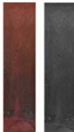
Figure 1. Example of a digitized and converted into 256 grey levels roof tile.
