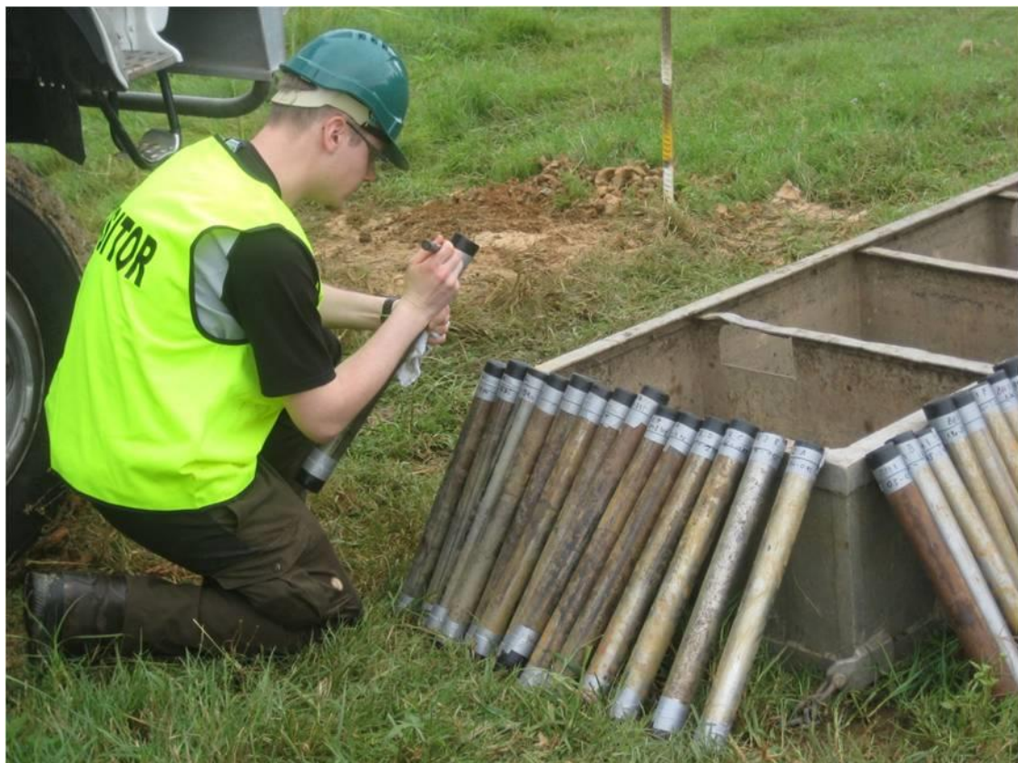
Figure 49 – Labelling of the undisturbed soil samples on site
