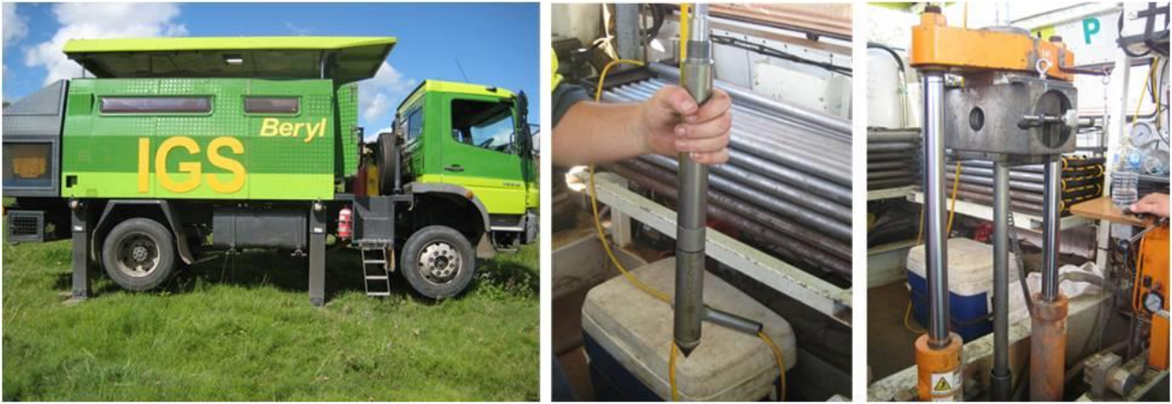
Figure 55 – CPT units at the field test site at Lawnton(vertical tests): truck-mounted CPT (left), cone (centre) and hydraulic jacking system (right)
