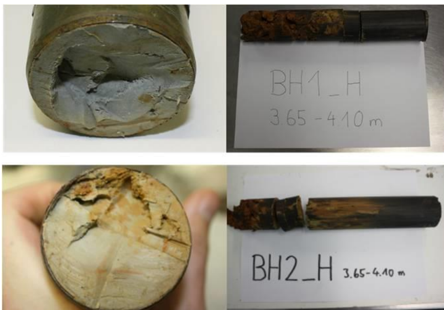
Figure 79 – Undisturbed soil samples of grey clay (-1.50 m to -6.50 m)
