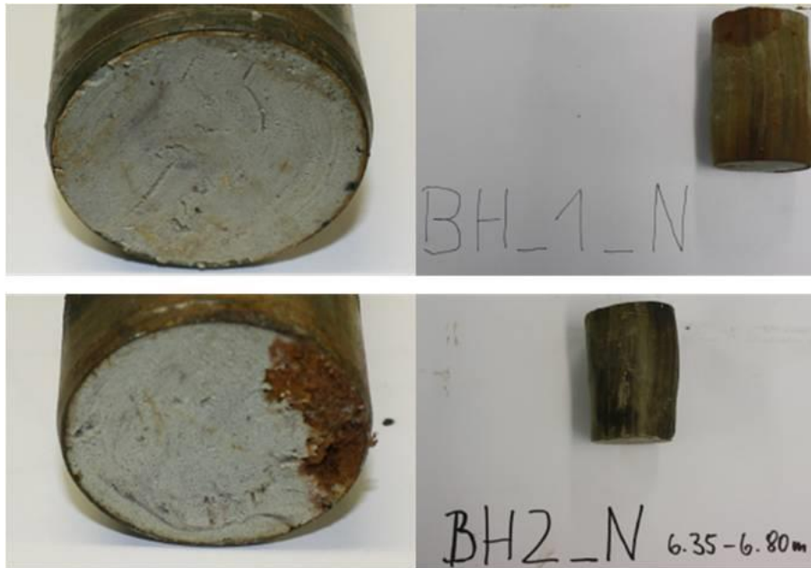
Figure 80 – Undisturbed soil samples of grey, sandy clay (-6.50 to -8.00 m)
