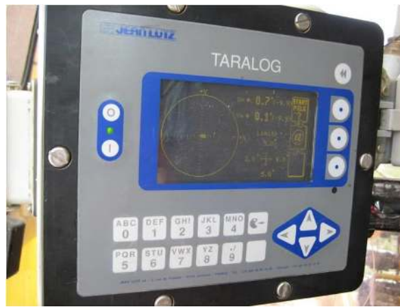
Figure 89 – Jean Lutz Taralog pile monitoring unit on site during the test execution
