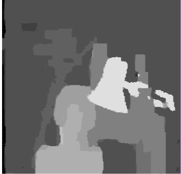
Figure 3. Disparity map generated for the Tsukuba data set using a GPU implementation of the algorithm by Felzenszwalb and Huttenlocher.
