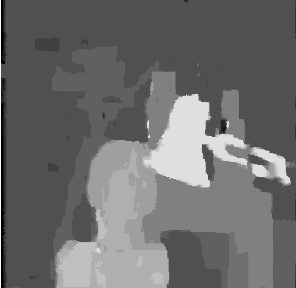
Figure 4. Disparity map generated for the Tsukuba data set using occlusion and edge information. Computed entirely on the graphics card.
