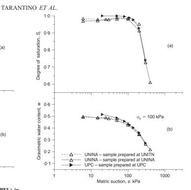
Fig. 4. Results from axis-translation oedometer (UNINA and UPC) in terms of (a) degree of saturation and (b) water content
