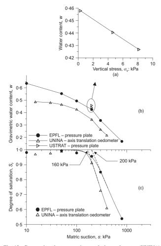
Fig. 12. Comparison between axis-translation oedometer (UNINA) and pressure plate (EPFL) and effect of contact pressure on water content (USTRAT)
