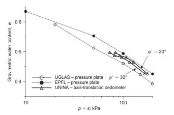
Fig. 5. Comparison of axis-translation data (pressure plate and oedometer) in the saturated range
