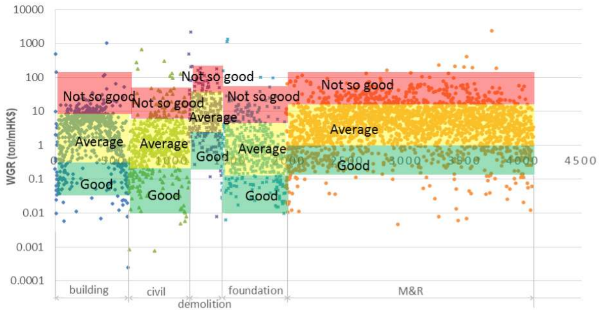
Fig. 11 Benchmarks of non-inert C&D waste management performance
