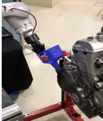
Figure 1-1: Oil Change Task - As one step in the Autonomous oil change task, the robot inserts the funnel into the engine.
