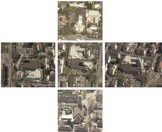
Figure 1. Church building in the benchmark area captured from all four oblique directions and the nadir view
