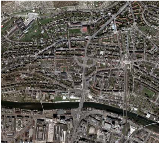
Figure 2. Ortho image of the test area in Zürich generated from oblique images looking northwards
