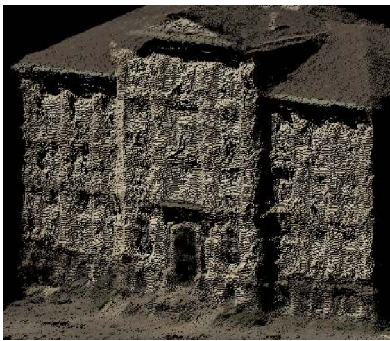
Figure 8. Point cloud of school building generated with SURE
