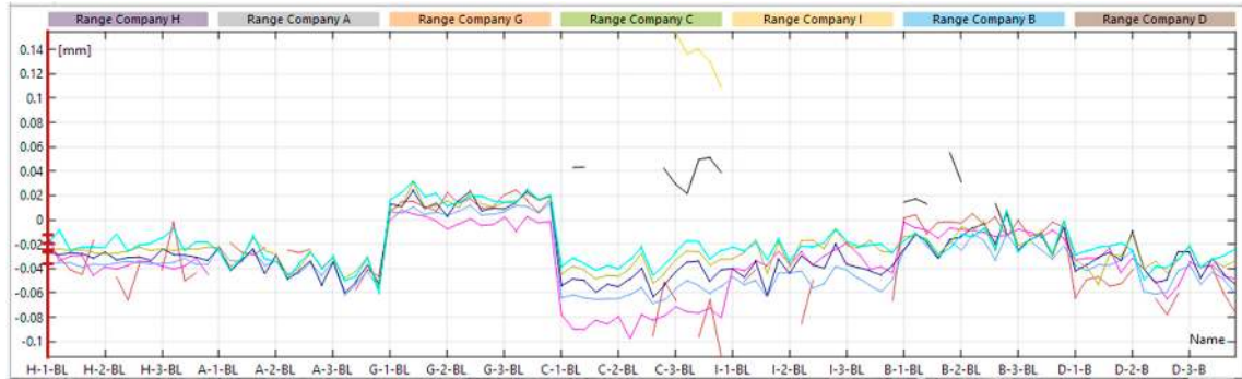
Figure 18. Deviation graph of the pin diameters compared to nominal CAD dimension produced with GOM Inspect for each pin from each company (in the graph, company F is referred to as company I).
