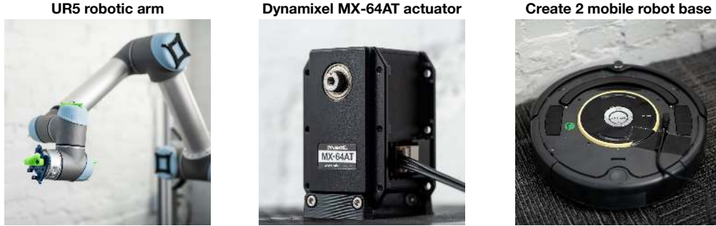
Figure 1: The robots used in this work: (left) Universal Robotics UR5 collaborative arms, (middle) Robotis MX-64AT Dynamixel actuators, and (right) iRobot Create2 mobile robot bases.
