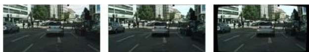
Fig. 6 Illustration of our proposed image corruptions. From left to right: Proposed noise model (severity level 4), PSF blur (severity level 3), and geometric distortion (severity level 1). Best viewed in color (Color figure online)
