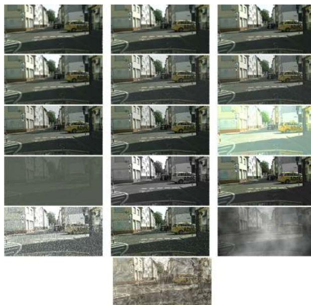
Fig. 2 Illustration of utilized image corruptions of ImageNet-C. First row (severity level 5 each): Motion blur, defocus blur, frosted glass blur. Second row (severity level 4 each): Gaussian blur, Gaussian noise, impulse noise. Third row (severity level 4, 4, 5 respectively): Shot noise, speckle noise, brightness. Fourth row (severity level 4, 2, 4 respectively): Contrast, saturate, JPEG. Fifth row (severity level 3, 3, 5 respectively): Snow, spatter, fog. Sixth row (severity level 5): frost
