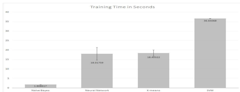
Figure 1: Average training time with marked standard deviation for each algorithm, collected over 100 passes.
