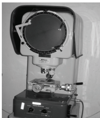
Figure 5. Profile projector machine.
