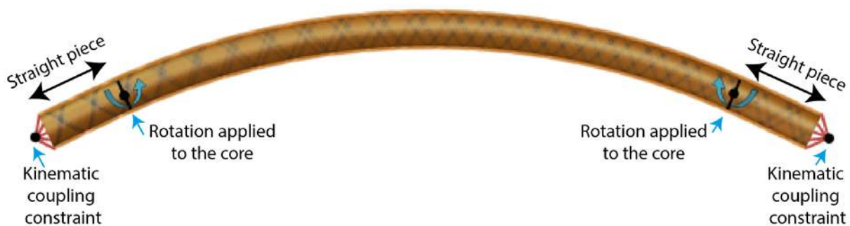
Figure 9. Boundary conditions for the cable bending model.
