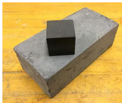
Figure 3. Photograph showing a cube sample used in the compression testing along side a full sized brick used in the LCA.
