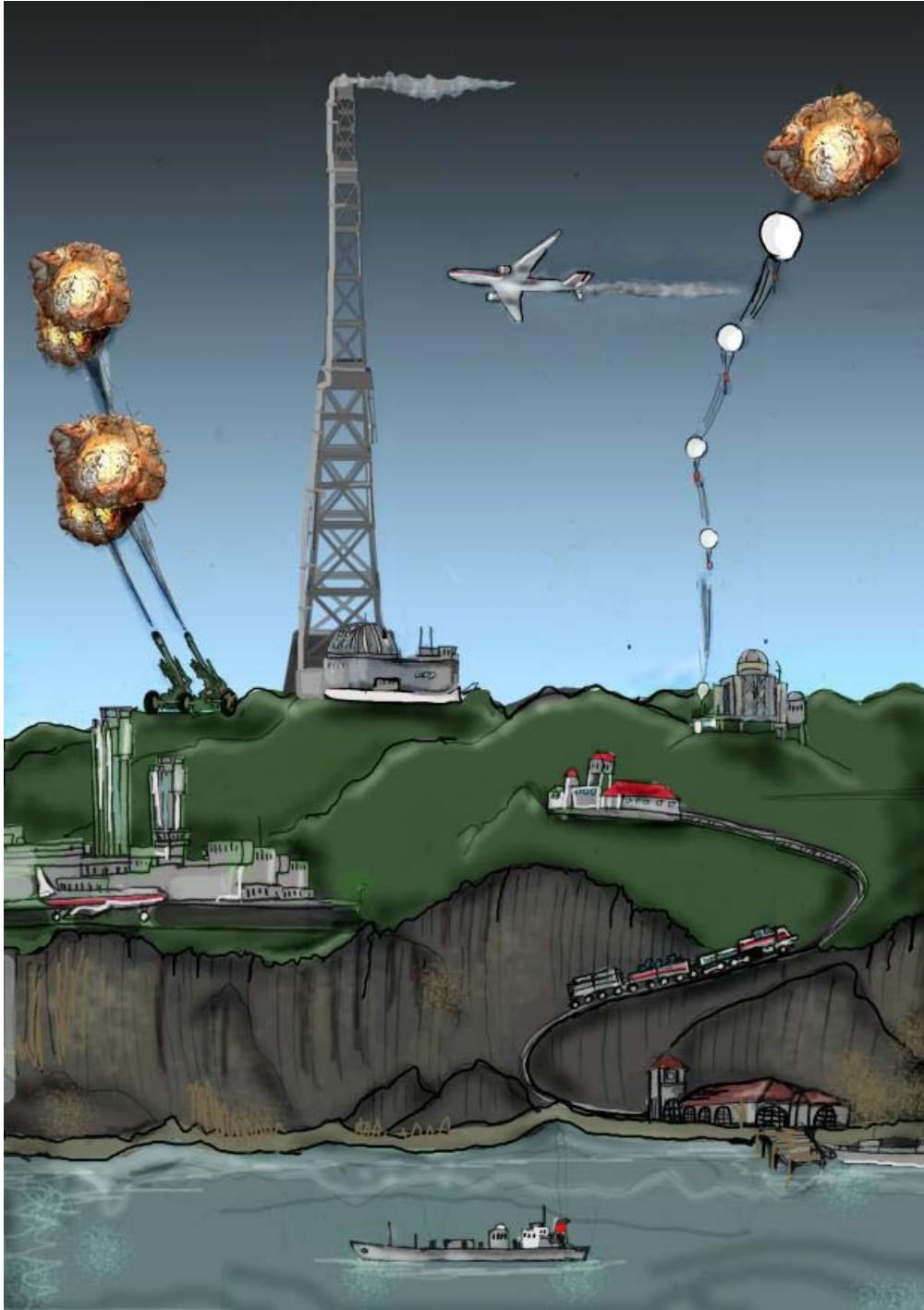
Figure 1. Proposed methods of stratospheric aerosol injection. A mountain top location would require less energy for lofting to stratosphere. Drawing by Brian West.
