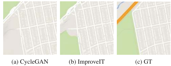
Figure 7: The result of CycleGAN and of using ImproveIT is shown here for the task of Sat2Map in comparison with the ground truth (GT). After fringe example detection, the input to the above image was sampled with Langevin dynamics. The result is the enhancement on the target domain, which can be visually noticed when comparing it to the GT.
