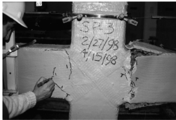
Figure 5–2 Retrofitted beam-column connection after testing (Mosallam, 2000)
