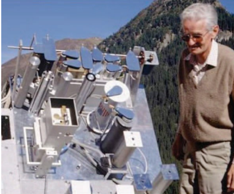
Figure 3-7. The World Standard Group of six absolute cavity radiometers is used to define the WRR or DNI measurement standard. Image by NREL
