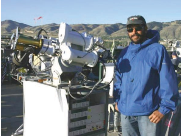
Figure 3-6. Multiple electrically self-calibrating absolute cavity radiometers mounted on solar trackers with control and data acquisition electronics. Image by NREL
