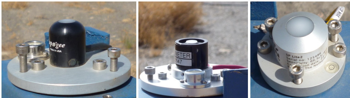
Figure 3-11. Selected photodiode sensors with different diffusor geometries. Photos from Stefan Wilbert, DLR
