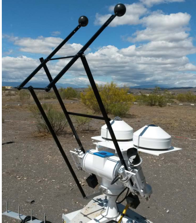
Figure 3-4. Pyrheliometer, a shaded pyranometer and a shaded pygeometer mounted on an automatic solar tracker. Photo from DLR
