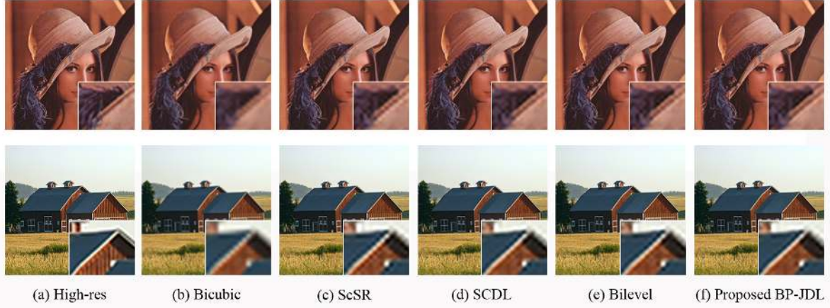
Figure 3. Visual comparison of factor of 2 super-resolution results. The upper row shows the SR results of the image Lena. The lower row shows the SR results of the image House.
