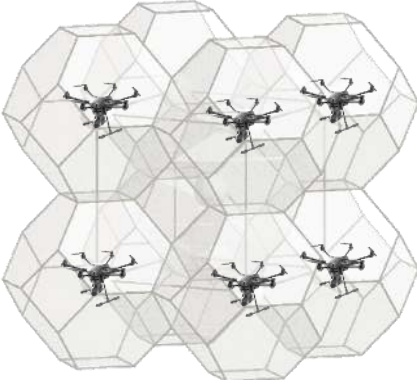
Fig. 4: Deployment of drone-BSs based on truncated octahedron cells.
