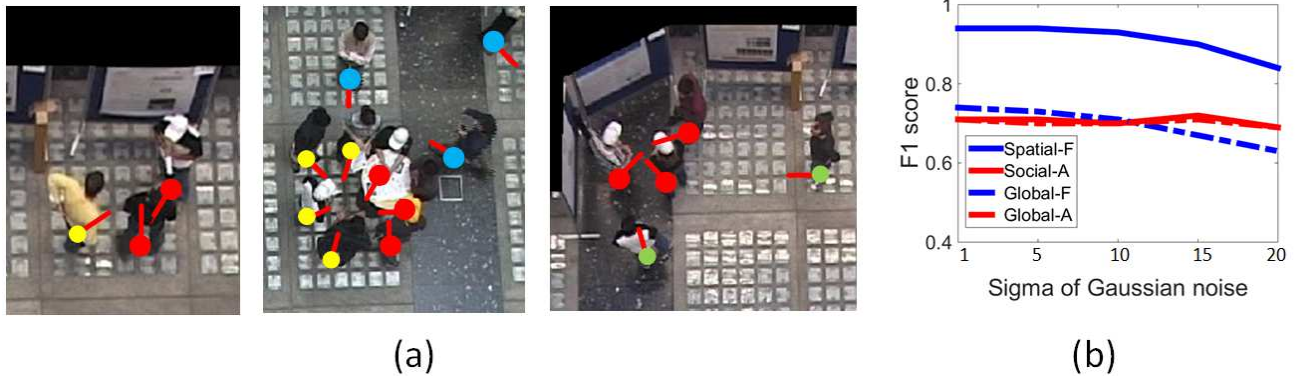
Figure 4. (a): example associate detection results: Red dots - members of an F-formation; red lines - body orientation; yellow dots - correctly detected associates; blue dots - correctly detected singletons; and green dots - missed associate detections. (b): F1 score of F-formation detectors spatial-F and global-F and associates detectors social-A and global-A with noisy test data.
