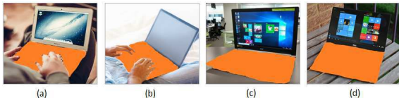
Figure 5: The shape of a part segmentation mask is related with its part state: (a) and (b) “keyboard is being used”, (c) and (d) “keyboard is not being used”. In (a) and (b), keyboards are occluded by human hands, thus the occluded area is excluded from the part segmentation mask.
