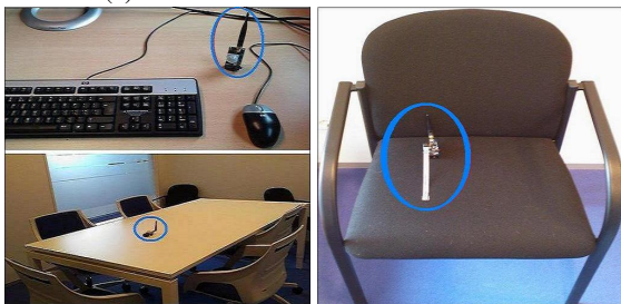
(b) Acoustic Sensors' Placement (c) Pressure Sensor Placement
