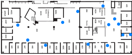
Figure 4: Testbed Topology. The figure shows the testing environment. The dots mark the locations of the GNU-Radio nodes.
