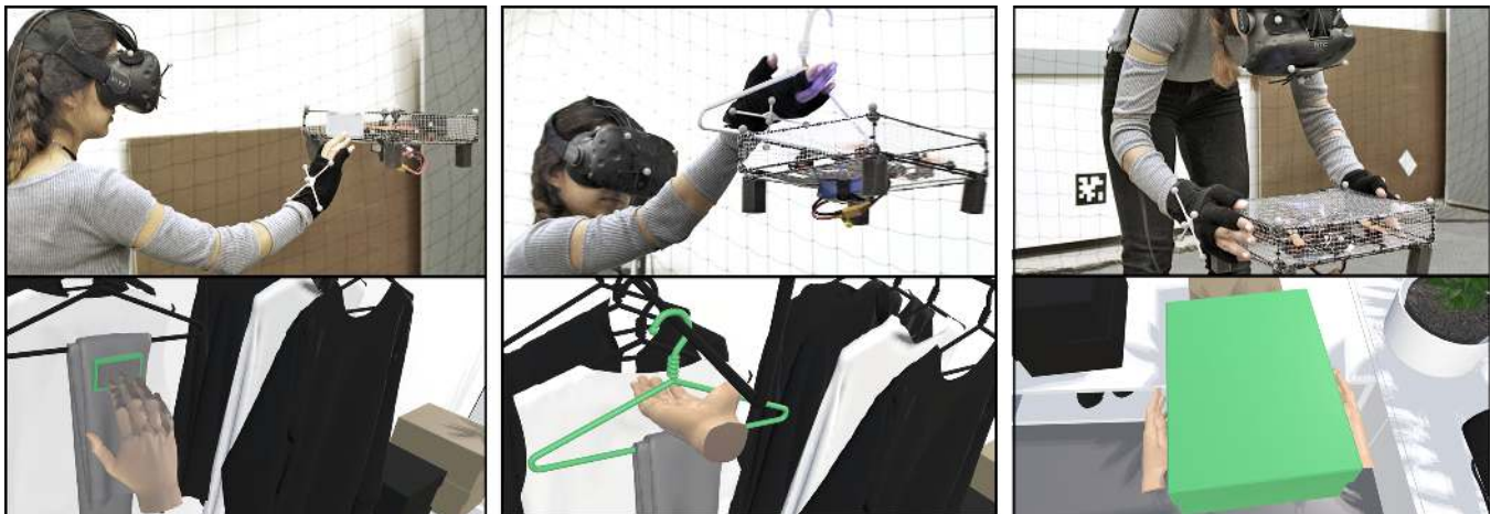
Figure 1: Haptic interactions using a quadcopter. Left: user touching fabrics attached to the quad for texture rendering. Middle: user picking up a physical hanger attached to the quad. Right: user picking up the turned off quad as a passive haptic device.
