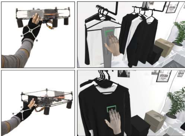
Figure 11: Texture rendering: user feeling the material of a scarf and a shirt.
