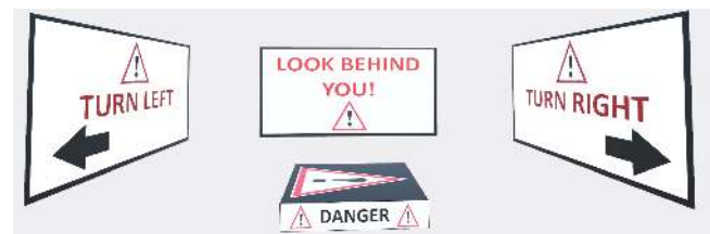
Figure 6: The emergency scene: the box in the center represents the current position of the quadcopter and warning signs pointing towards the quad are placed around the user.
