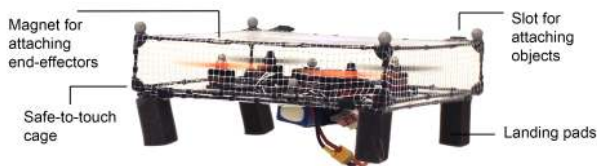
Figure 8: Safe-to-touch quadcopter with the protective cage.
