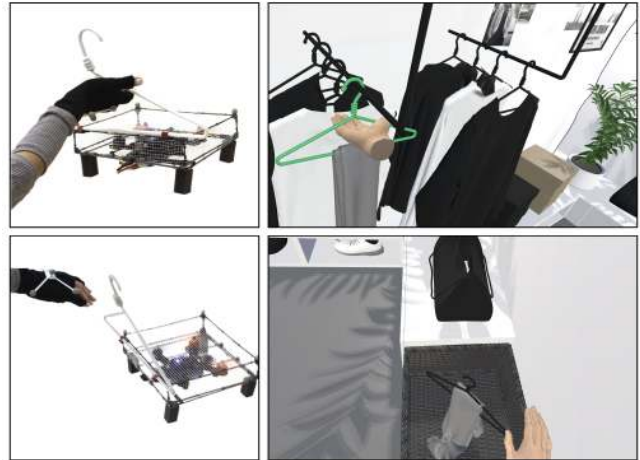
Figure 12: Animating passive props: user picking up a hanger and dropping it in the shopping basket.
