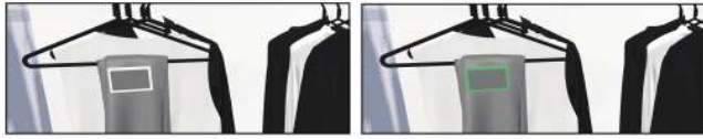
Figure 7: Upon the quad’s arrival the patch is highlighted in green, indicating that the user can touch the virtual object.
