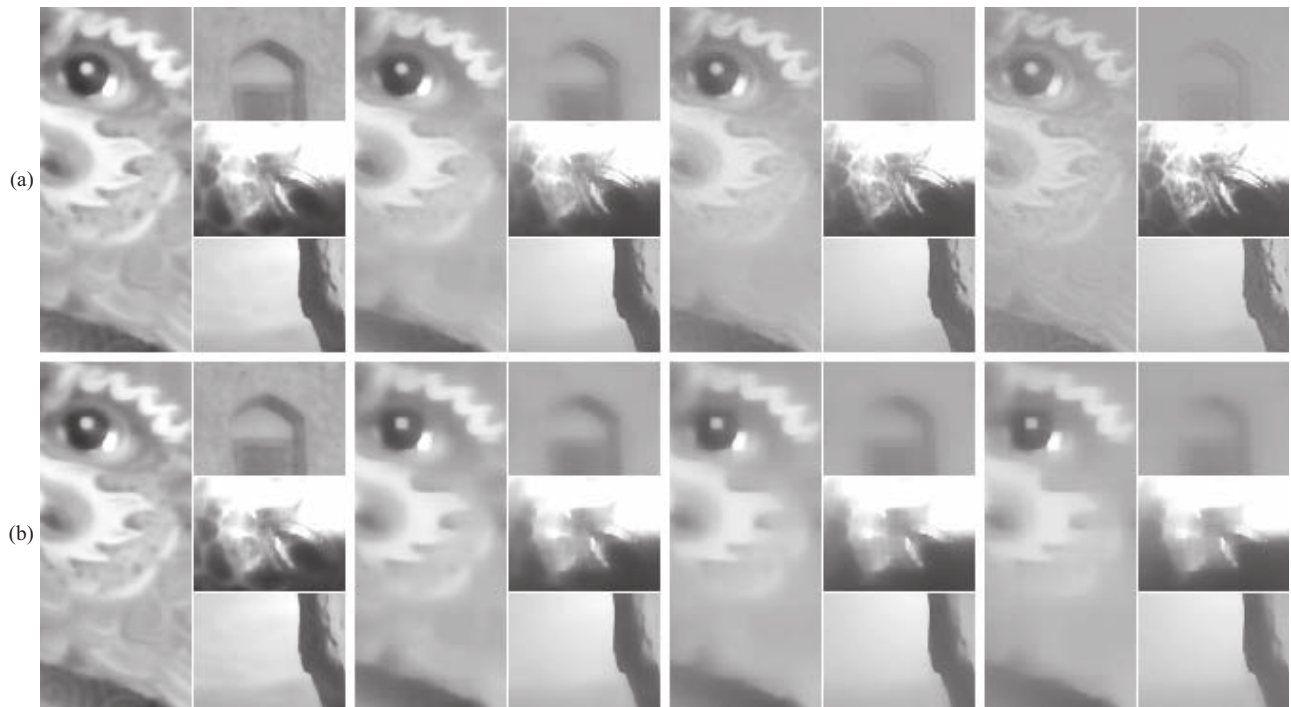
Fig. 10. (a) Application of the bilateral filter and (b) BEEPS to the cutouts from Fig. 8. The bi-exponential spatial filter takes the contra-decay \lambda \in \{0.5, 0.8, 0.9, 0.95\} , from left to right. The standard deviation of the Gaussian range filter is kept constant, with \sigma = 50 .
